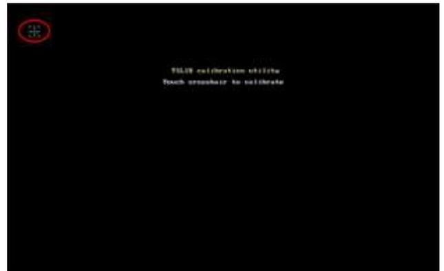
※ **During the correction, please do perform the operation according to the positions of crosses. Otherwise, the touching panel will be unable to**
